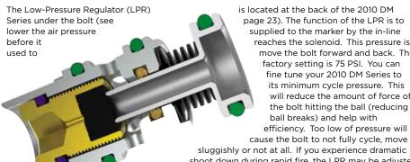
is located at the back of the 2010 DM page 23). The function of the LPR is to supplied to the marker by the in-line reaches the solenoid. This pressure is move the bolt forward and back. The factory setting is 75 PSI. You can fine tune your 2010 DM Series to its minimum cycle pressure. This will reduce the amount of force of the bolt hitting the ball (reducing ball breaks) and help with efficiency. Too low of pressure will
