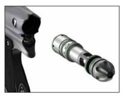
ports in the bolt and out the front of the bolt to propel the ball. When the bolt is in the forward position, the inside bolt stem O-ring prevents the flow of air from continuously flowing through the marker when the bolt is forward. This helps the marker shoot much more efficiently.
